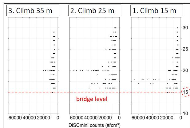
Figure 5: Vertical concentration profiles of ultrafine particles measured by the instrumented octocopter in 15m, 25m, 35m distance to the bridge, repectively
