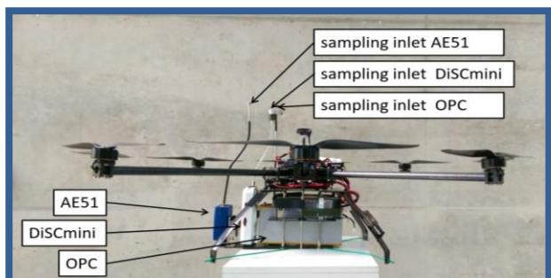
Figure 4: Octocopter with measurement instruments
