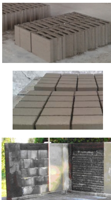
Fig. 1. Concrete blocks and building bricks, vibropressed and hydraulic strengthened, obtained from bottom ash and cement
