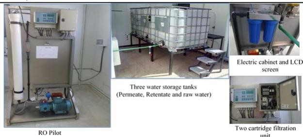
Fig. 2: Reverse osmosis plant installed on the site of UDES laboratory
