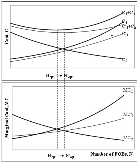
**Fig. 1a.** Dependence of partial costs  $C_1$  and  $C_2$  on the number of FOBs  $N$  and shifting of  $N_{opt}$  in case of introducing into the network a new large floating platform, properly equipped.
