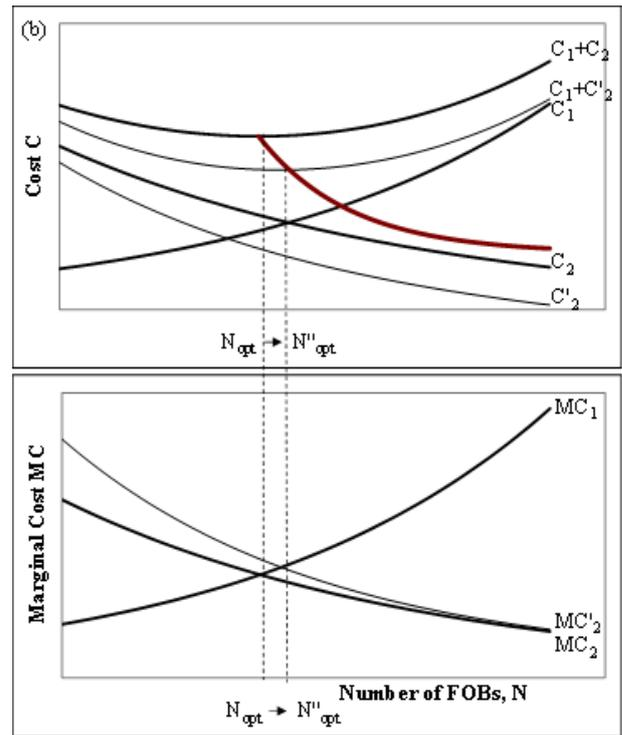
**Fig. 1b.** Dependence of partial costs  $C_1$  and  $C_2$  on the number of FOBs  $N$  and shifting of  $N_{opt}$  in case that the whole project is further subsidized with funds supporting environmental policy making and regional development; the thick line in the upper diagram is the locus of  $C_{min}$  points, when subsidization changes.
