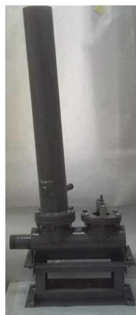
Fig.5 The ram pump used for tests.
