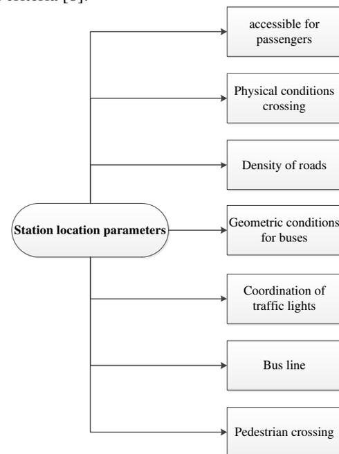
Fig. 8 Parameters of station location
