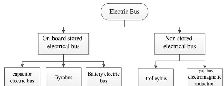
Fig. 2 Electrical bus types
