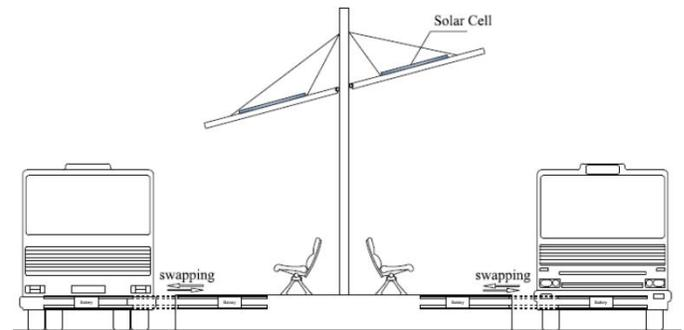
Fig. 11 Battery replacement mechanism
