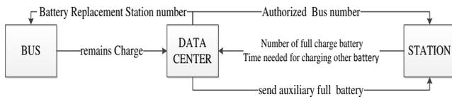
Fig. 9 Mechanism of system
