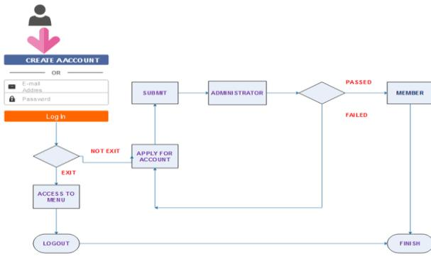
Fig.4 Login diagram for a fresh application.
