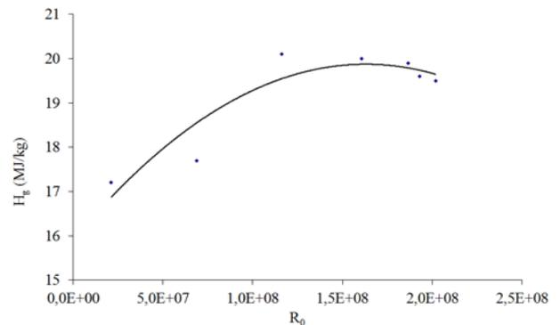
Fig.4: Gross heat of cimbustion vs severity factor.
