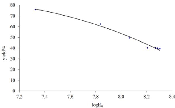
Fig.3: Torrefied cotton mass yield as affected by severity factor in logarithmic form.
