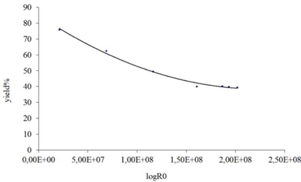
Fig.2: Torrefacted cotton mass yield as affected by severity factor.
