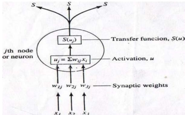
Fig. 5 The standard diagram of a generalized node in an artificial neural network
