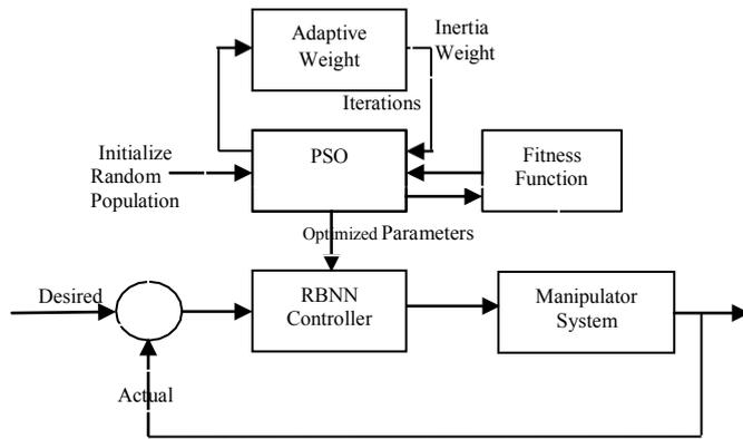
Fig. 4: Working of the proposed control scheme
