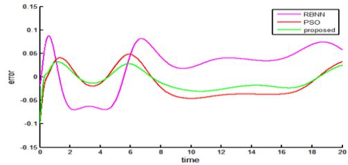
Fig. 9: Tracking error for Joint 2
