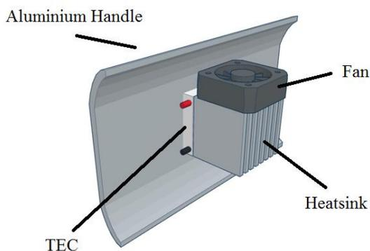
Fig.2 – Thermal module design.
