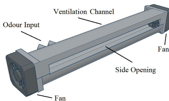
Fig.3 – Air channel design.
