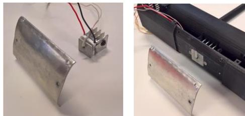
Fig.6 – Thermal module assembly.
