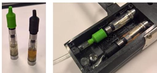
Fig.7 – Clearomizers assembly.
