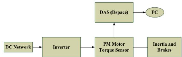
Fig. 3 Testing bench for motor measurements
