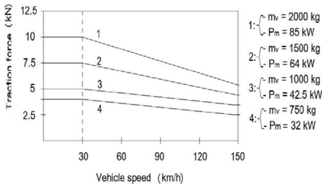
Fig. 1 Traction characteristics.
