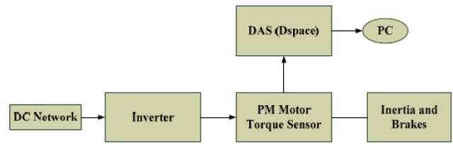
Fig. 3 Testing bench for motor measurements
