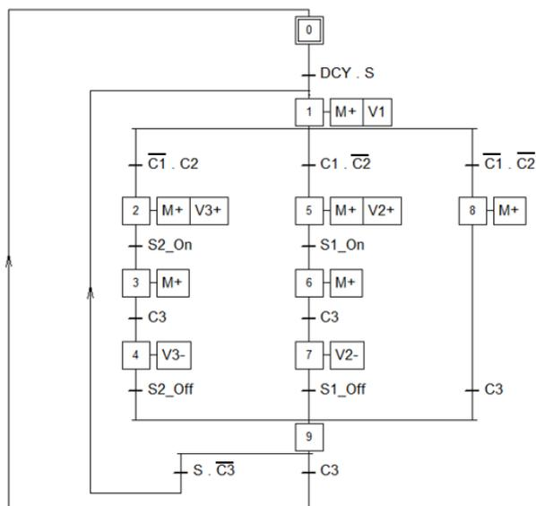
Fig.3: GRAFCET of the sorting station operation
