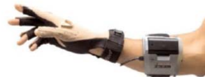
Fig. 2 Cyberglove II flex sensors based MCS (Cyberglove Systems image)
