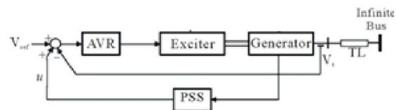
Fig.1 Block schematic diagram of the proposed SMIB Power system controller
