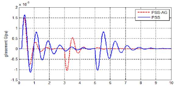
Fig.4 functioning system in the nominal régime used of TBB-500 connected to a long line with,  $H_{\infty}$ -PSS,PSSPID(robustness tests) (Ug, Pe ,glissement ,delta)
