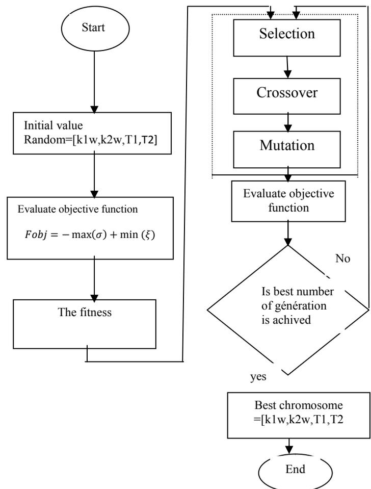
Fig.4 The algorithm for the computation of PSS-PID parameters using genetic algorithm.
