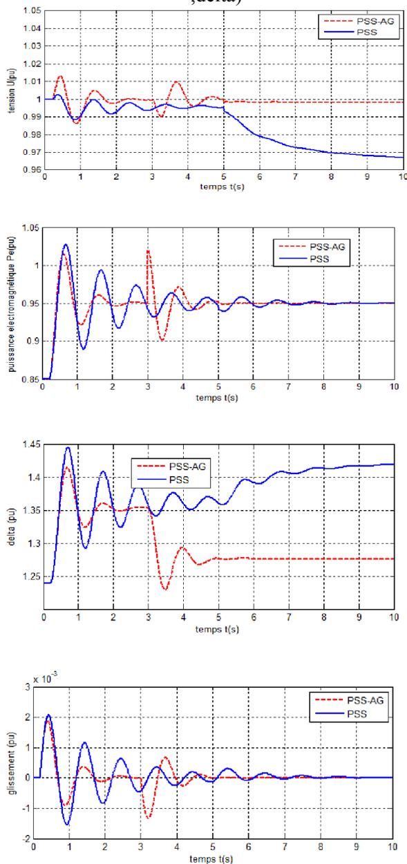
**Fig.6** functioning system in the over-excited used of TBB-500 connected to a long line with,  $H_{\infty}$  - PSS,PSSPID(robustness tests) ( $U_g$ ,  $P_e$ , glissement,  $\delta$ )
