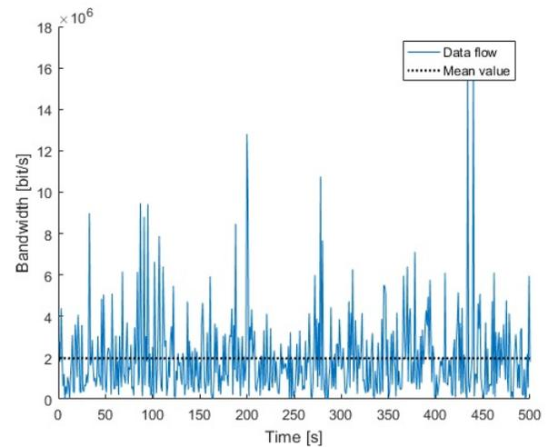
Figure 3: Example of the first accepted data flow time variation.
