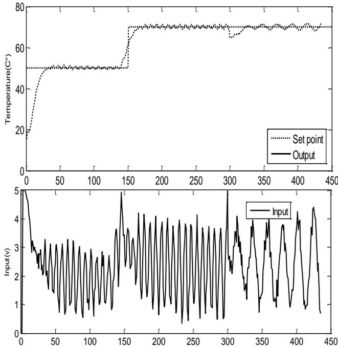
Fig. 5. Closed-loop results obtained with FPC
