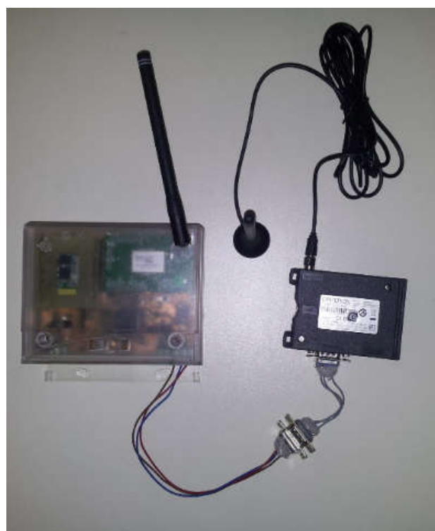
Fig. 5. The connection between MI-MDCU and GPRS modules.
