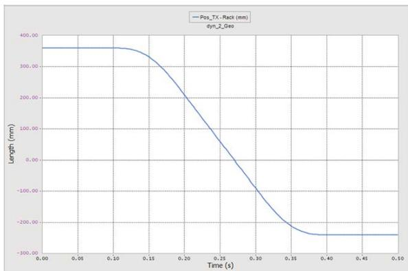
Fig. 3 Analysis result of displacement of rack gear translation
