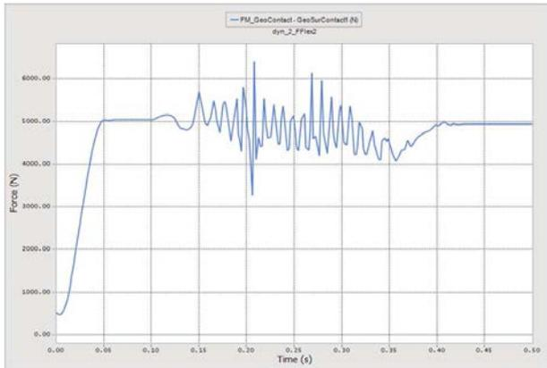
(a) Contact force between rack and pinion
