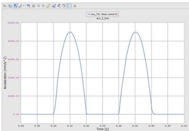
Fig. 4 Analysis result of acceleration of rack gear
