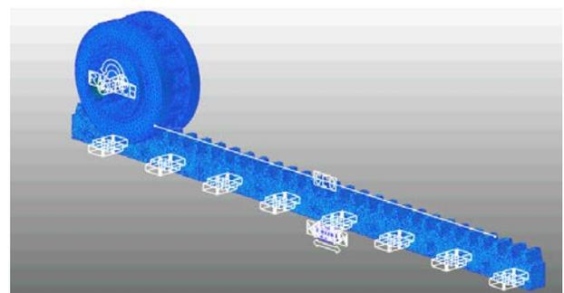
Fig. 12 Analysis lattices of rack & pinion
