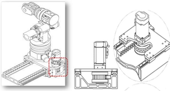
Fig. 1 The fusion reducer module for robot system
