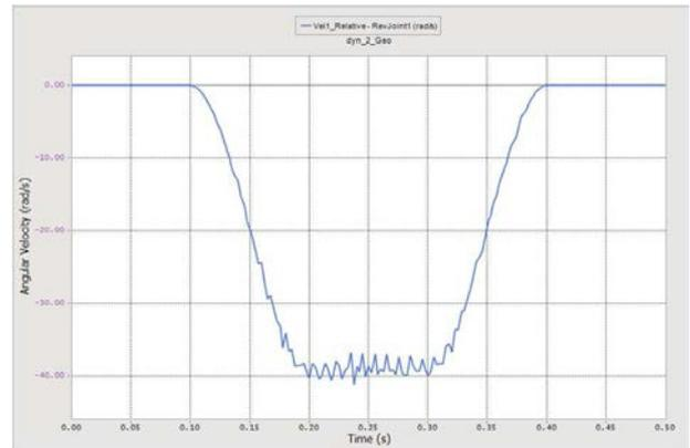
Fig. 5 Analysis result of angular velocity of pinion gear
