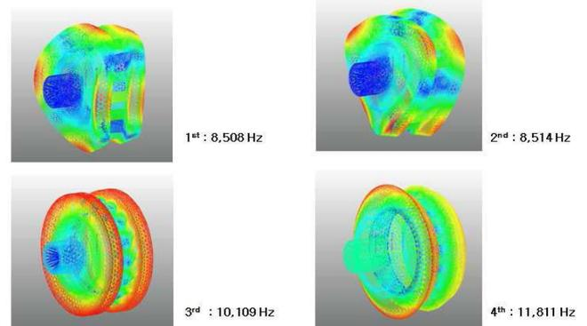
Fig.10 Analysis result of natural frequency of pinion gear
