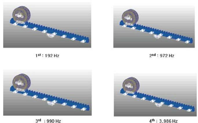
Fig.11 Analysis result of natural frequency of rack and pinion gear
