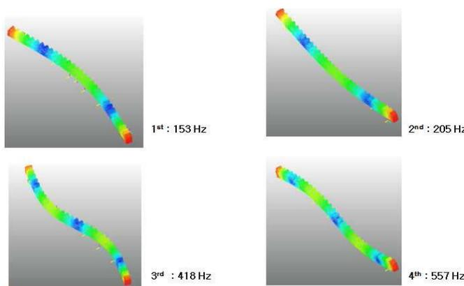
Fig.9 Analysis result of natural frequency of rack gear
