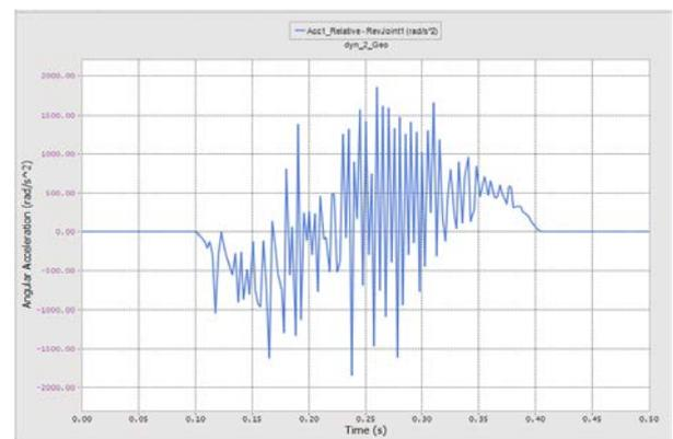
Fig. 6 Analysis result of angular acceleration of pinion gear
