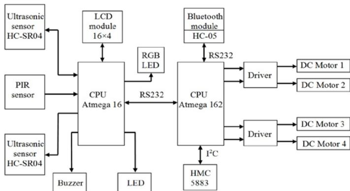
Fig. 1. The block diagram of the robot control system
