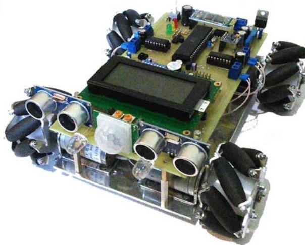
Fig. 2. Autonomous mobile robot on wheels rolikonesuschih
