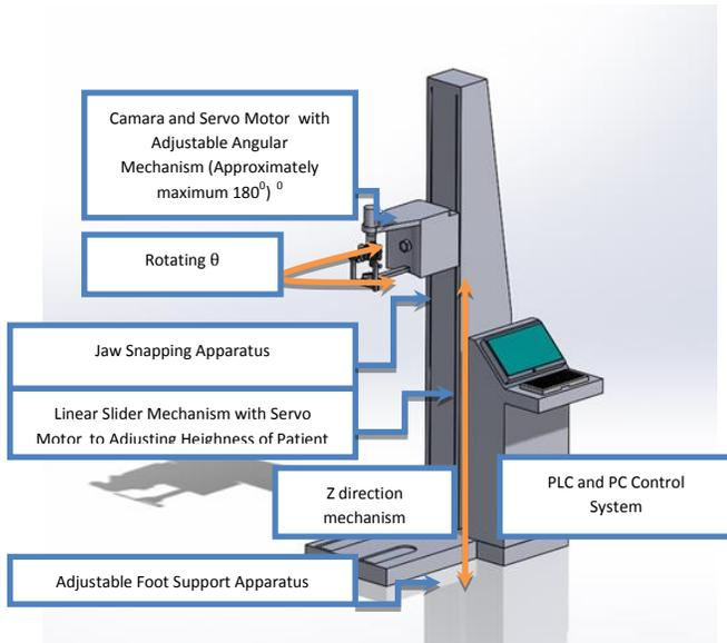
Fig. 2 (b). The proposed fully automated system and main elements
