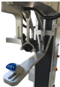
Fig. 3. Camara and chin position apparatus
