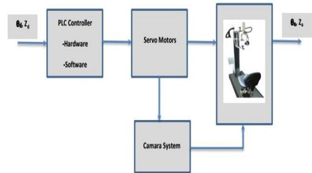
Fig.5. Block diagram of position control process
