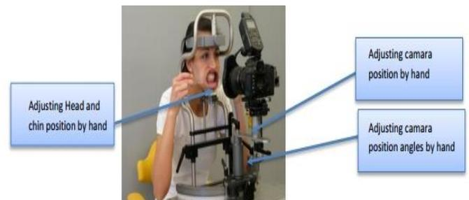
Fig.1. View of manually positioning system and description
