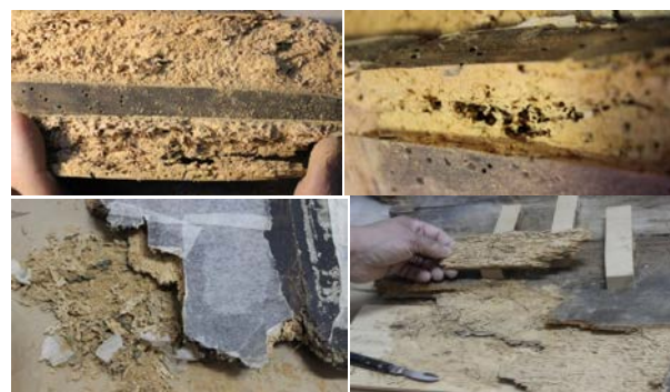
Fig 1. Deep degradation of wooden support of icons
