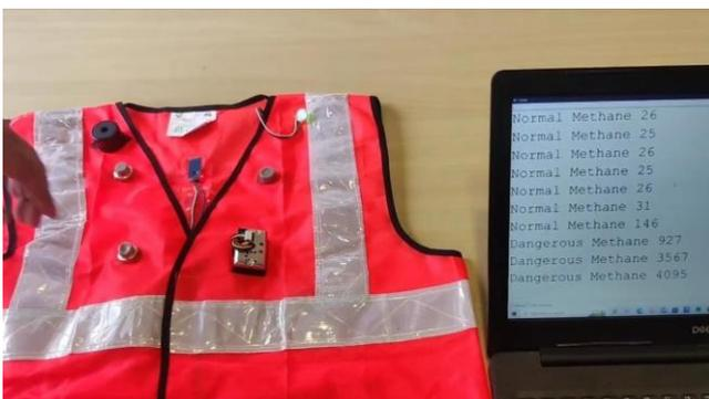
Fig 7 Gas Sensor Measurement
