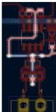
Fig. 11. A CAN-BUS interface circuit that does not comply with EMC standards
