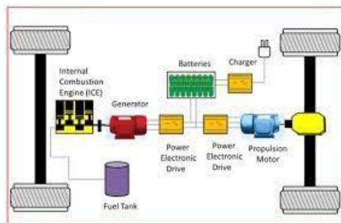
Fig. 1. Hybrid electric vehicle, Series-Parallel [8]
