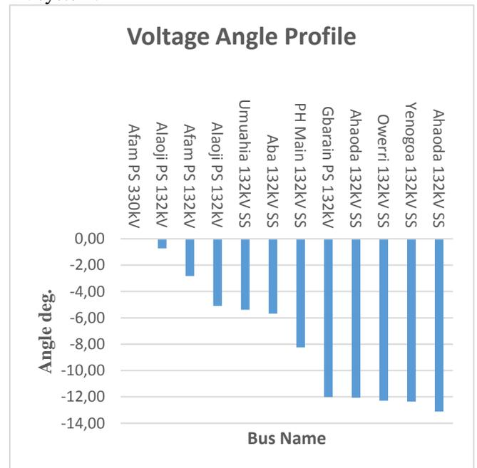
Figure 5: Bar chart of Voltage angles without PV system.
