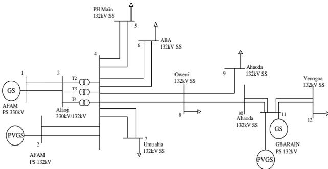
Figure 3: Single Line Diagram of the modified network
