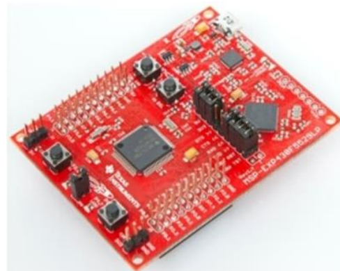
Fig.2 MSP430F5529LP \mu\text{C} board
