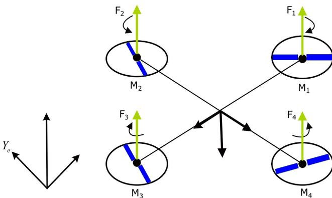
Figure 1: The quadrotor UAV with four rotors.
