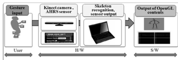
Fig. 8 System configuration
