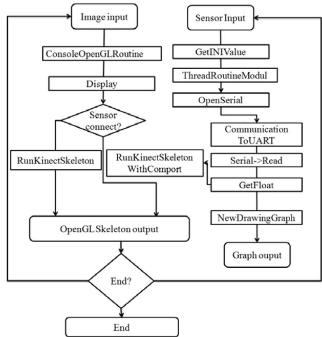
Fig. 3 HMC software flow chart
