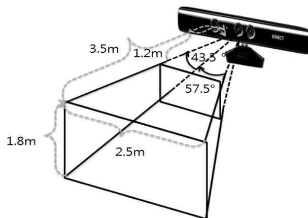
Fig. 3 Range of Kinect camera
