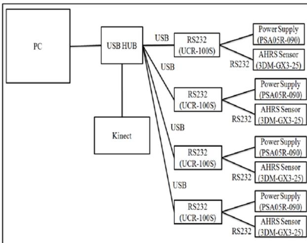
Fig. 10 H/W flow block diagram
