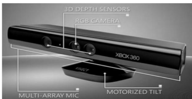
Fig. 2 Windows-based Kinect camera
