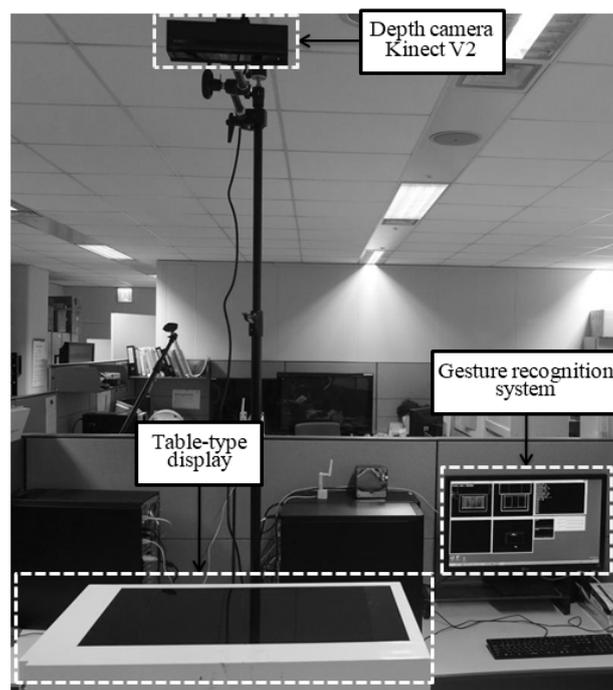
Fig. 1 Schematic view of the system
