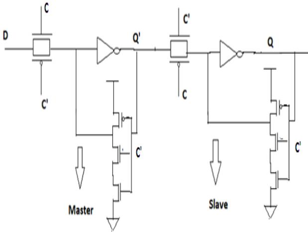
Fig. 8 Proposed D flip-flop
