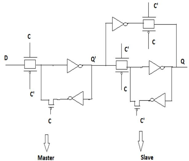
Fig. 7 Push pull isolation D flip-flop [1]
