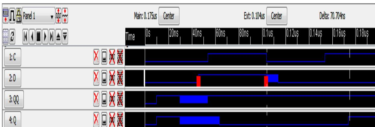
Fig.10 Waveform of proposed D flip-flop
