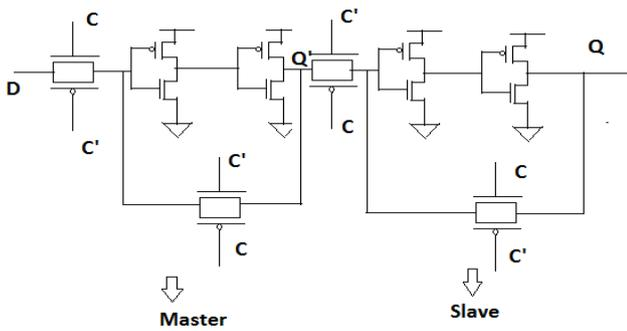
Fig.1 Transmission Gate Flip-flop [1]
