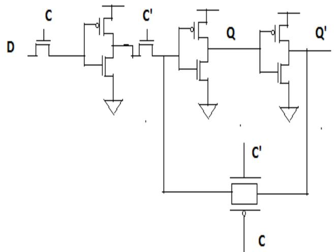
Fig. 4 Ten transistor SET D flip-flop [1]
