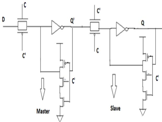
Fig. 8 Proposed D flip-flop
