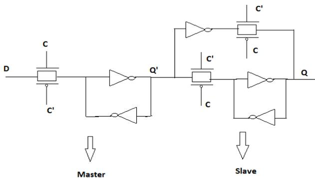
Fig.6 Push pull D flip-flop [1]
