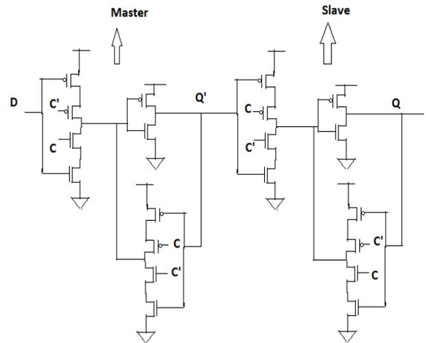
Fig.3 Clocked CMOS D flip-flop [1]
