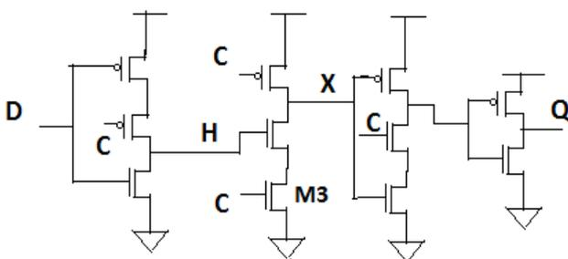
Fig.2 True Single Phase Clock D Flip-Flop [1]
