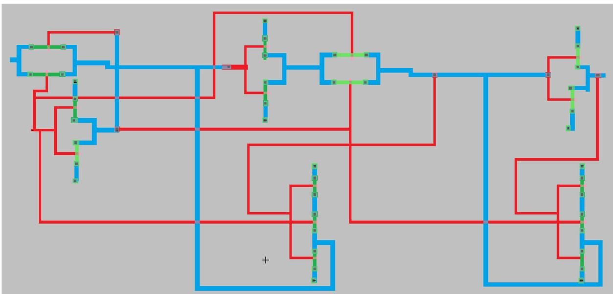
Fig. 9 Proposed D flip-flop Layout
