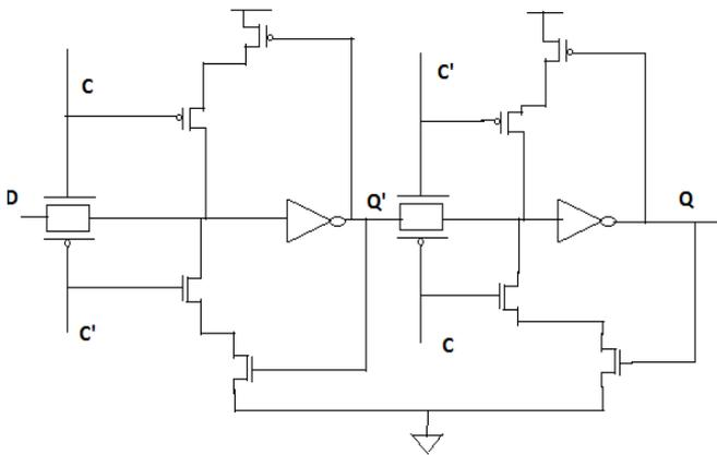
Fig. 5 Low power D flip-flop [1]
