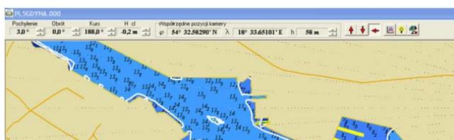
Fig. 8. Edition window for inserting parameters of projection and speed of camera in motion
