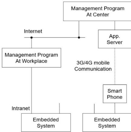
Fig. 2 The dataflow of the oyster output management system
