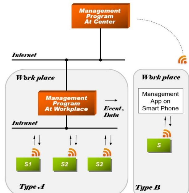
Fig. 1 The overview of oyster output management system
