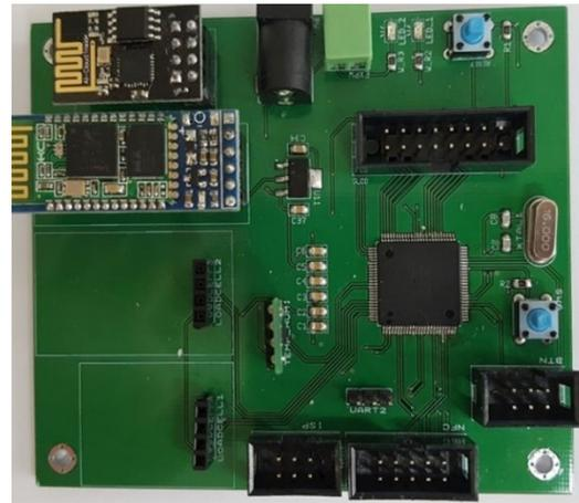
Fig. 10 Developed PCB of the embedded system
