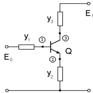
Fig. 6. One-stage transistor amplifier.
