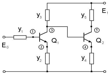
Fig. 8. Two-stage transistor amplifier.
