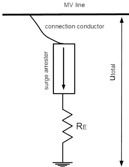
**Fig. 2** Connection of surge arrester to a MV line
