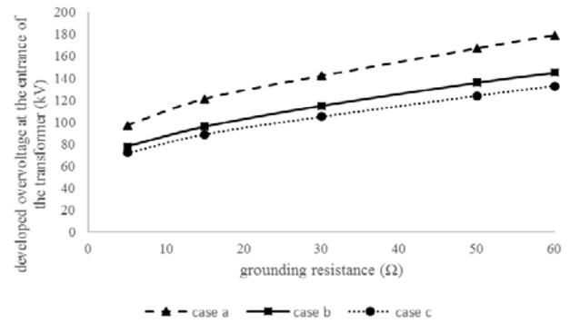
**Fig. 4** The developed overvoltages at the entrance of the transformer in comparison to the grounding resistance for the examined cases
