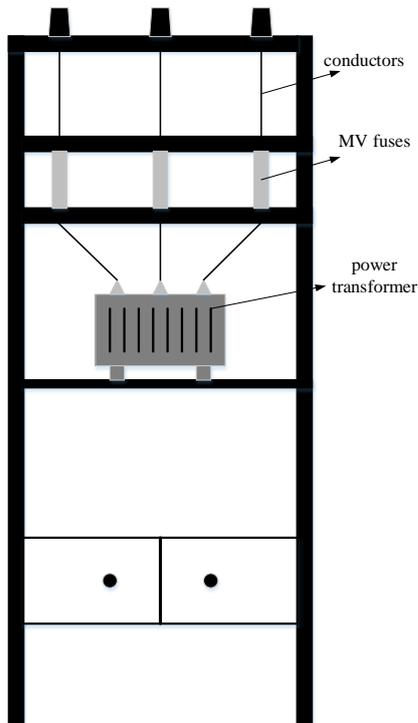
**Fig. 1** Configuration of a distribution substation
