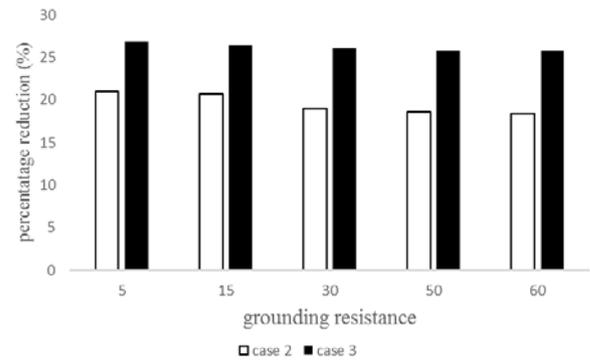
**Fig. 5** The percentage reduction of the developed overvoltages for Cases 2 and 3 compared to Case 1
