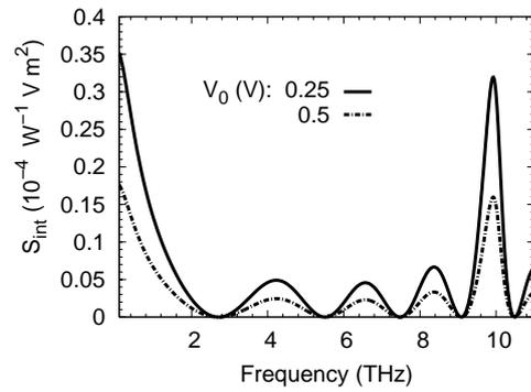
Figure 7: Intrinsic Responsivity  $S_{int}$  as functions of ac voltage component  $V_0$ . With  $\omega_0 = 10$  GHz,  $L = 400$  nm,  $\nu = 3 \times 10^{12}$  s $^{-1}$  and carrier concentration  $n_0 = 8 \times 10^{17}$  cm $^{-3}$ .
