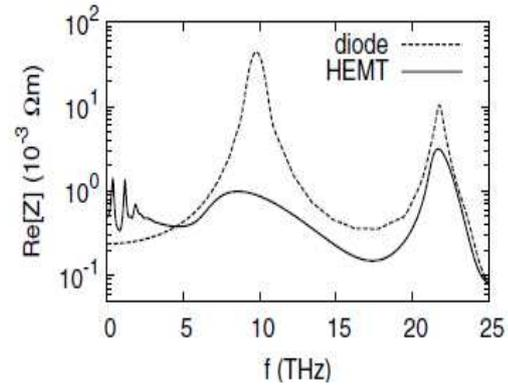
Figure 4: The real part of small-signal impedance calculated for the diode (dashed line) and HEMT transistor (solid line) under the constant-drain-current operation.
