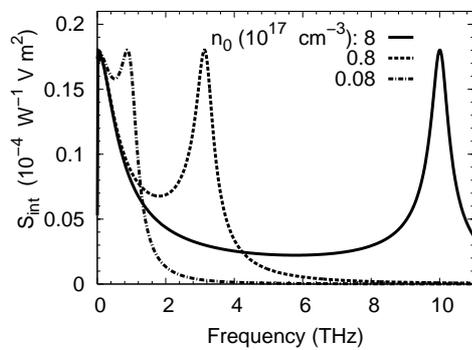
Figure 6: Intrinsic Responsivity  $S_{int}$  calculated for different electron concentration  $n_0$  with  $L = 400$  nm and  $V_0 = 0.25$  Volt.
