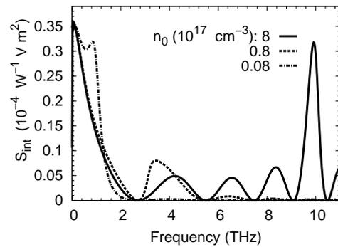
Figure 8: Intrinsic Responsivity  $S_{int}$  calculated for different electron concentration  $n_0$  with applied voltage  $V(t)$ .
