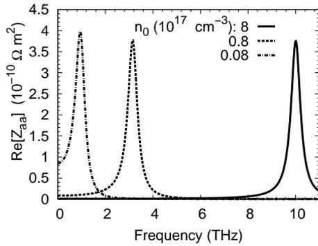
Figure 3: Real part of impedance as functions of the frequency for the reported electron concentration. With  $L = 400$  nm,  $\nu = 3 \times 10^{12}$  s $^{-1}$ .
