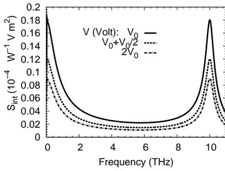
Figure 5: Intrinsic responsivity  $S_{int}$  for different fixed values of the voltage  $V$  corresponding to different phases of the ac component  $V(t) = V_0 + V_0 \cos(\omega_0 t)$  ( $\omega_0 t = 0, \pi/3, \pi/2$ ). With  $V_0 = 0.25$  V,  $L = 400$  nm,  $\nu = 3 \times 10^{12}$  s $^{-1}$  and electron concentration  $n_0 = 8 \times 10^{17}$  cm $^{-3}$ .
