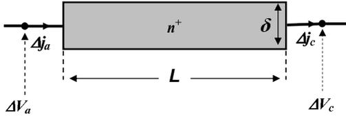
Figure 1: Structure representation of an high doped unipolar diode  $n^+$  of length  $L$  and thickness  $\delta$ . The amplitudes of the anode and cathode are  $\Delta V_a$  and  $\Delta V_c$  respectively.
