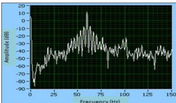
Fig. 7 Frequency spectrum of the motor current damaged
