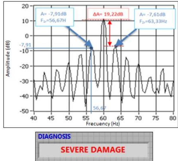
Fig. 8. Motor test report damaged
