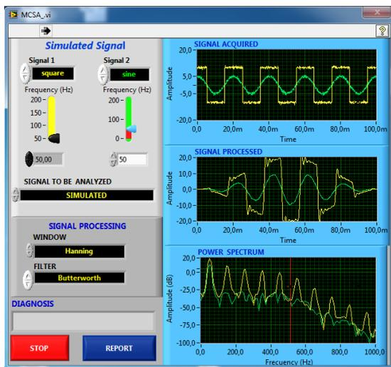
Fig. 3 Front panel
