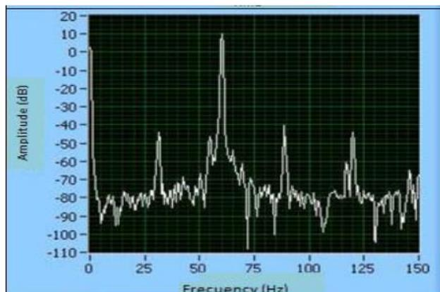
Fig. 10 Frequency spectrum of the current healthy motor
