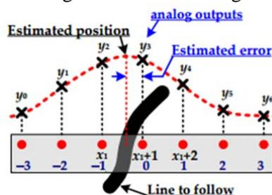
Fig.1 Line detection via quadratic interpolation [11]
