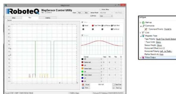
Fig 4. MagSensor control utility GUI for the magnetic guide sensor configuration
