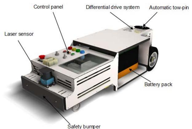
Fig. 2 CAD model of the AGC
