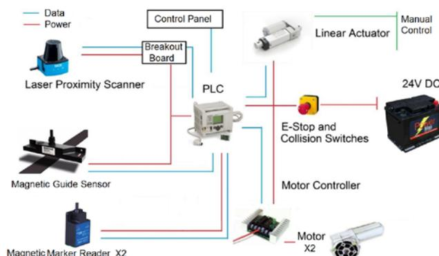
Fig. 3 AGC controller architecture
