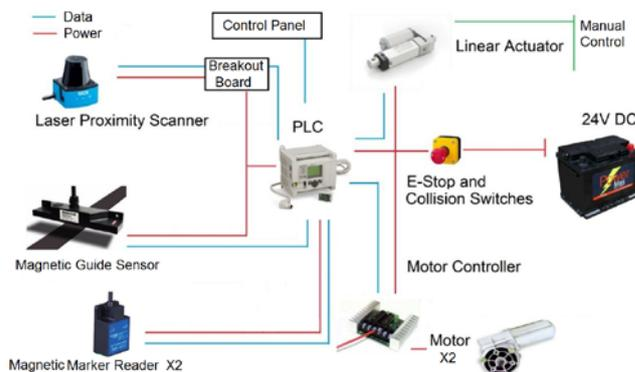
Fig. 3 AGC controller architecture
