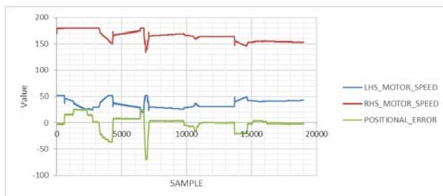
Fig. 5 Error signal and motor commands during operation
