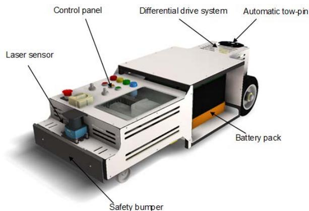
Fig. 2 CAD model of the AGC
