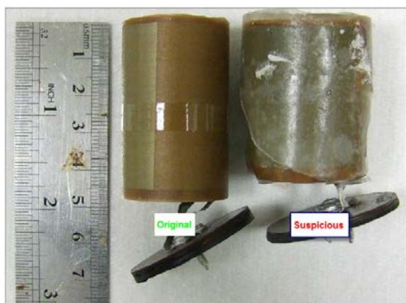
Fig. 6 Encapsulated capacitors for foil reel measurement
