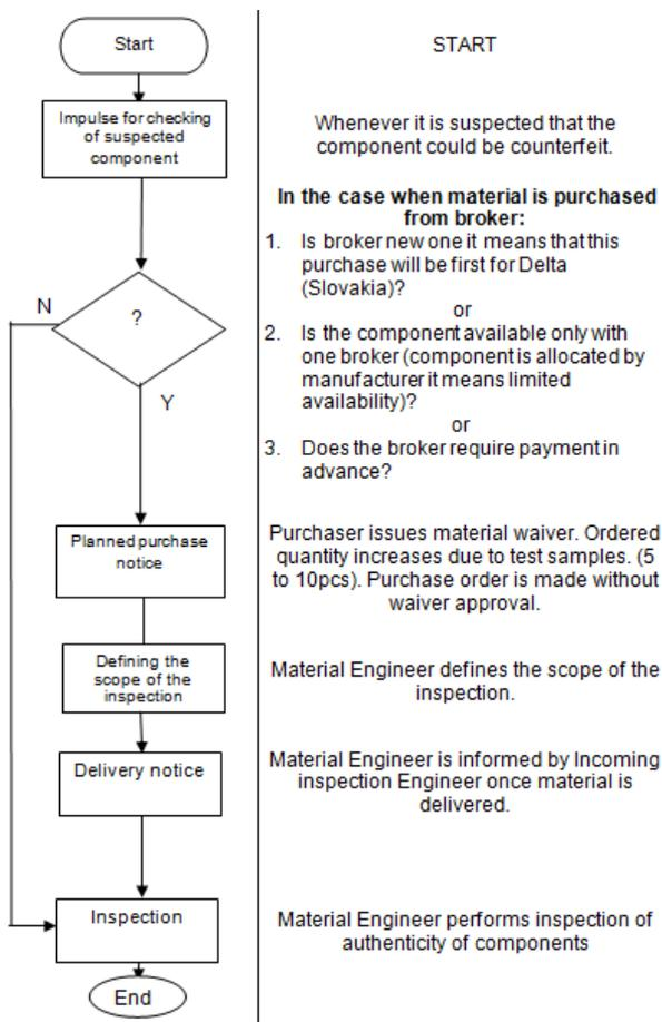
Fig. 1 Flow chart for counterfeit component detection
