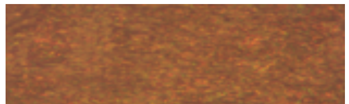
Fig 4 –Structure of copper surface with a porosity of 0.24% after immersion in PGC for 6 hours and kept inside an air sealed box for two days, as viewed under metallurgical microscope in 40 X magnifications. The change in structure and formation of nano porous gold is seen through the microscopic view. Further heating for 2 minutes reduces the resistance to 0.12Ω
