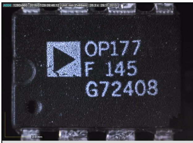
Fig. 51 OP177 by AD package marking in oblique lighting.
