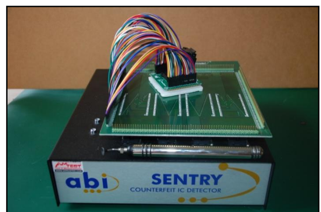
Fig.6 Counterfeit IC detector with a variant of general-purpose contact adaptor.
