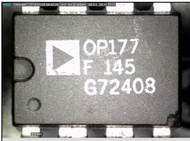
Fig.50 OP177 by AD package marking in direct vertical lighting.
