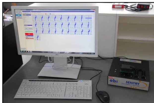
Fig. 8 ASA component pin print comparative evaluation workstation.
