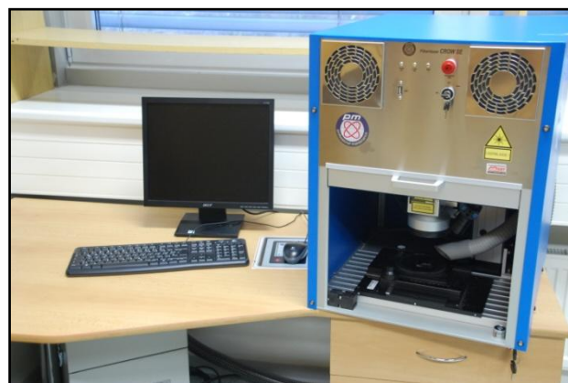
Fig.7 Fiber laser workstation with decapsulation and marking compartment open.
