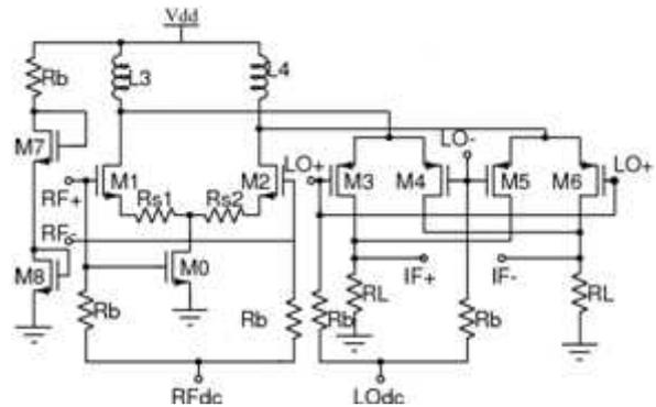
Fig.7: Folded Gilbert Mixer with  $R_{s1}$  and  $R_{s2}$
