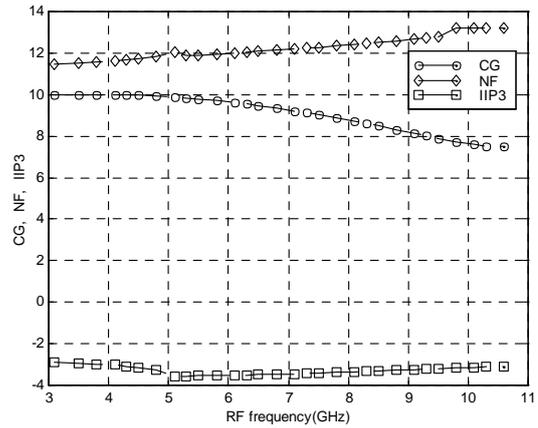
Fig.4: Plot of RF frequency versus CG, NF, IIP3
