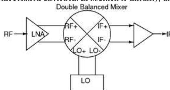
Fig. 2: Block diagram of Receiver Front end
