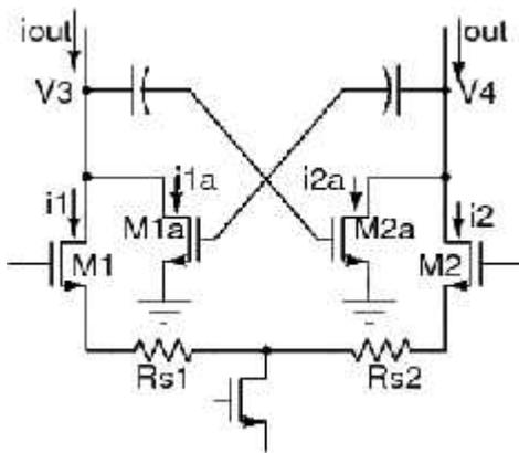
Fig. 9: Cross section of mixer showing auxiliary transistor
