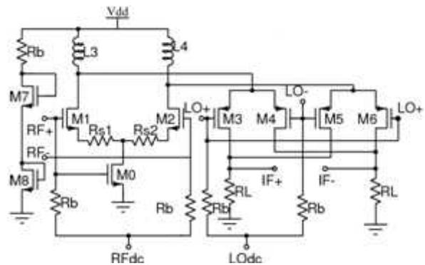
Fig.7: Folded Gilbert Mixer with  $R_{s1}$  and  $R_{s2}$
