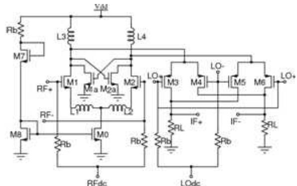
Fig. 8: Complete schematic of proposed mixer
