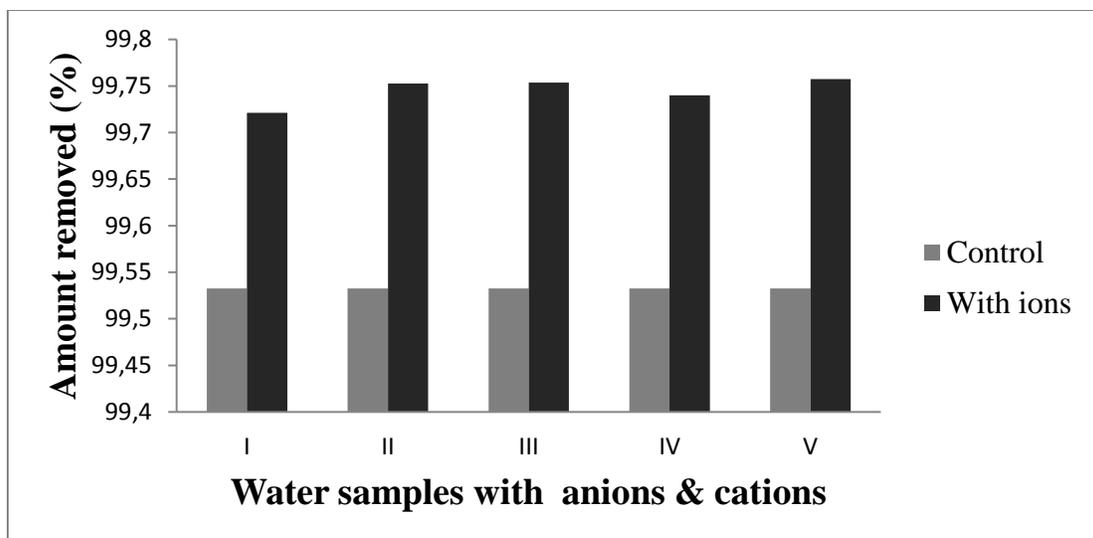
Fig. 11. Influence of Co-ions (anions & cations) towards  $\text{PO}_4^{3-}$  adsorption on allophane soil adsorbent
