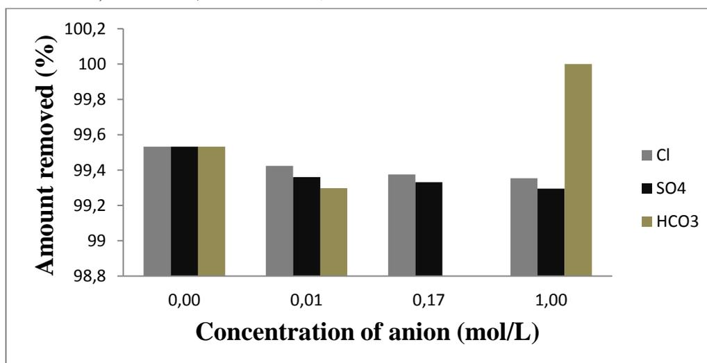
Fig. 10. Influence of Co-ions (anions) towards  $\text{PO}_4^{3-}$  adsorption on allophane soil adsorbent
