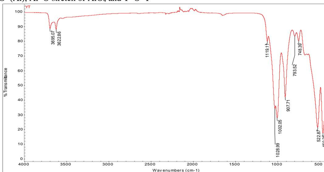
Fig. 3. FTIR spectrum of allophone soil adsorbent
