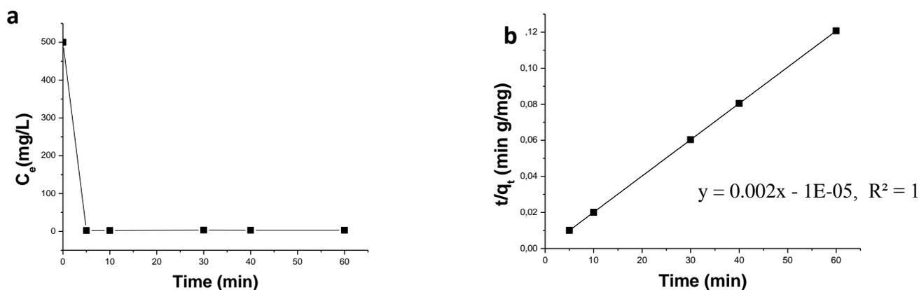
Fig. 7. **a** Influence of contact time **b** Linearized Pseudo-second order kinetic model towards  $\text{PO}_4^{3-}$  adsorption on allophane soil adsorbent
