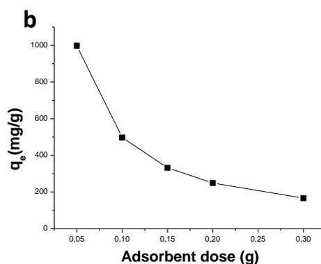
Fig. 9. a Influence of pH b Influence of adsorbent dose towards  $\text{PO}_4^{3-}$  adsorption on allophane soil adsorbent
