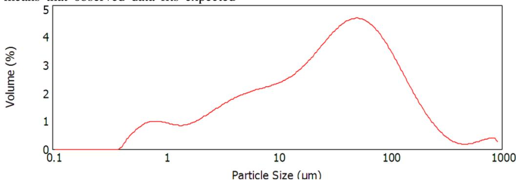
Fig. 1. Particle size distribution curve of allophane soil adsorbent
