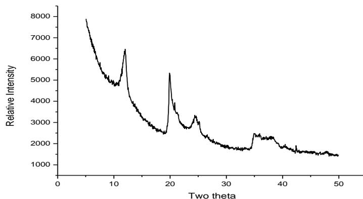
Fig. 4. XRD pattern of allophane soil adsorbent
