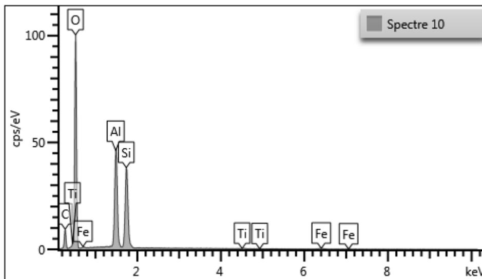
Fig. 2. Elemental composition of allophone soil adsorbent
