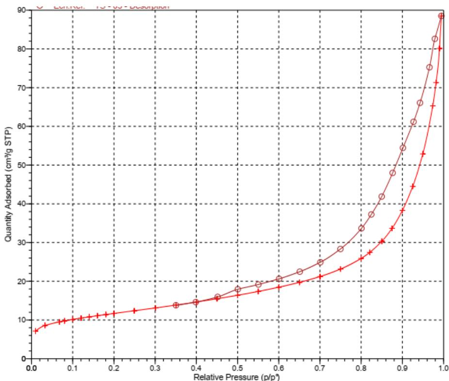
Fig. 6. Nitrogen adsorption-desorption isotherm of allophane soil adsorbent
