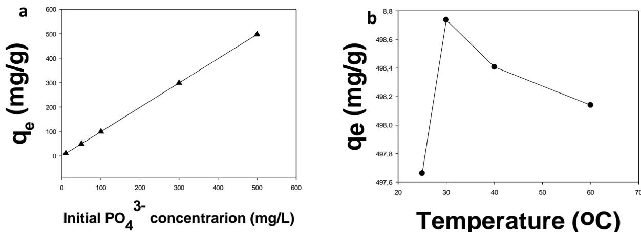
Fig. 8. **a** Influence of initial concentration (initial  $\text{PO}_4^{3-}$  concentration 10-500 mg/L, adsorbent dose 0.1g, pH 6.8, temperature of 25°C, contact time of 10 minutes) **b** Influence of temperature (initial  $\text{PO}_4^{3-}$  concentration 500 mg/L, 0.1 g adsorbent, pH 6.8, contact time 10 minutes) towards  $\text{PO}_4^{3-}$  adsorption on allophane soil adsorbent
