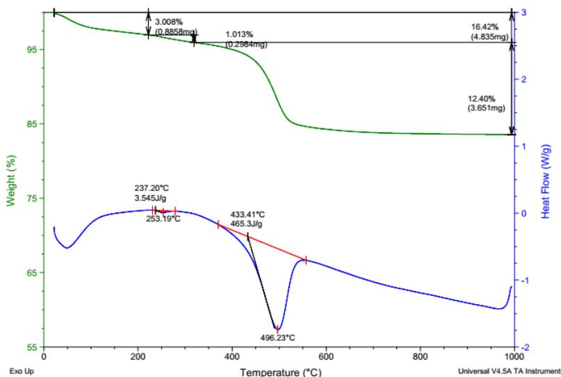
Fig. 5. TGA-DSC curves of allophane soil adsorbent
