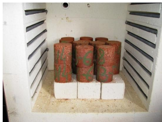
Figure 3a. Thermal treatment. Burning
