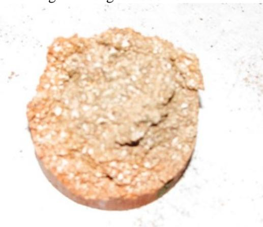
Figure 4. Appearance of a broken sample showing no carbon traces
