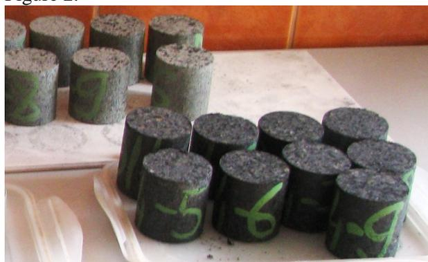
Figure 2. Samples obtained through semi-dry pressing
