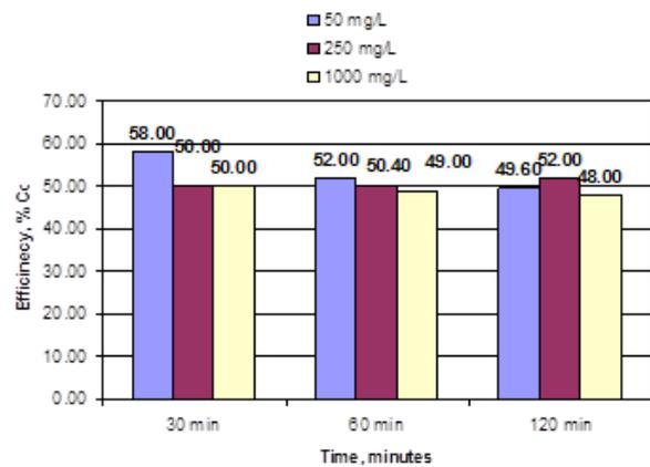
Fig. 8: Removal efficiency for Cd onto Fe<sub>3</sub>O<sub>4</sub> at different concentrations
