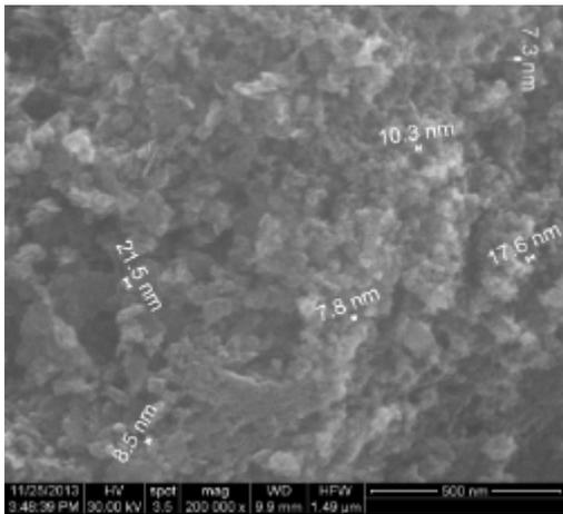
Fig. 4: SEM image with the nanoparticles dimensions for 200000x magnification
