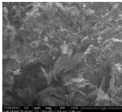
Fig 3: SEM image with acicular and spherical aspect of magnetite at 100000x magnification
