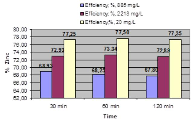
Fig. 7: Removal efficiency for Zn onto Fe<sub>3</sub>O<sub>4</sub> at different concentrations
