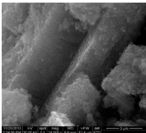
Fig 2: SEM image of the nanoparticles (nanomagnetite) at magnification of 24000x
