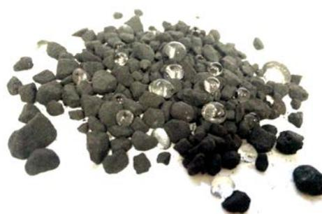
Figure 8 - Photo of water droplets on the surface of the hydrophobic sand
