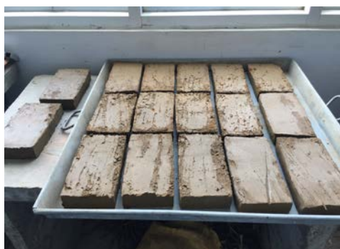
Fig.1 Modified Fly Ash-Bricks with Sago Husk
