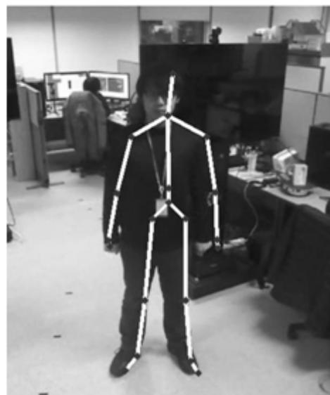
Fig. 16 Skeleton model extracted from the image input by the 3D camera
