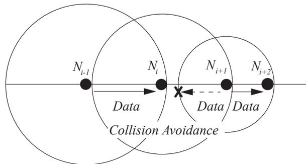
Figure 2: Collision Avoidance with Hop-by-Hop Shortening Multihop Transmission Route.
