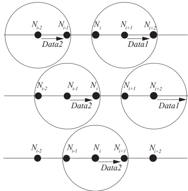
Figure 1: End-to-End Throughput in Conventional Wireless Multihop Transmissions.
