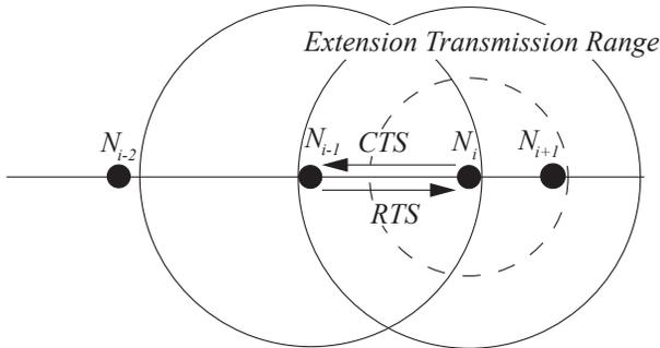
Figure 5: CTS Transmission with Higher Transmission Power.
