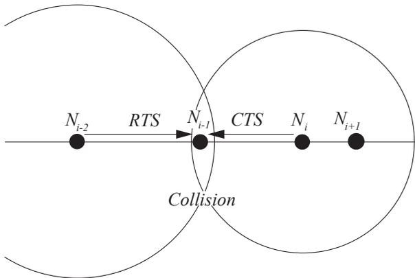
Figure 6: Possible Collision between RTS and Power-Controlled CTS.
