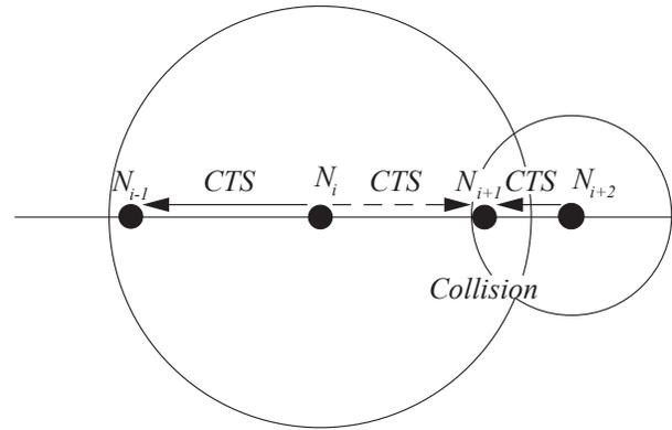
Figure 7: Possible Collision between Power-Controlled CTSs.
