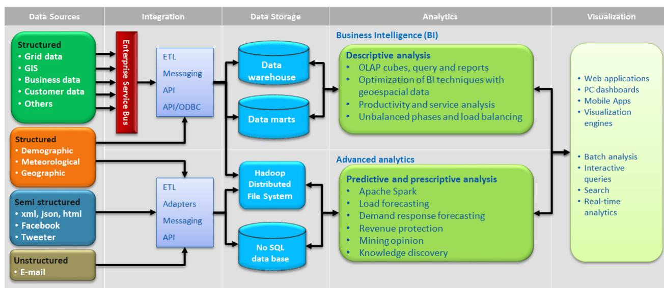
Figure 2. The conceptual architecture of the analytics platform for electric distribution data.
